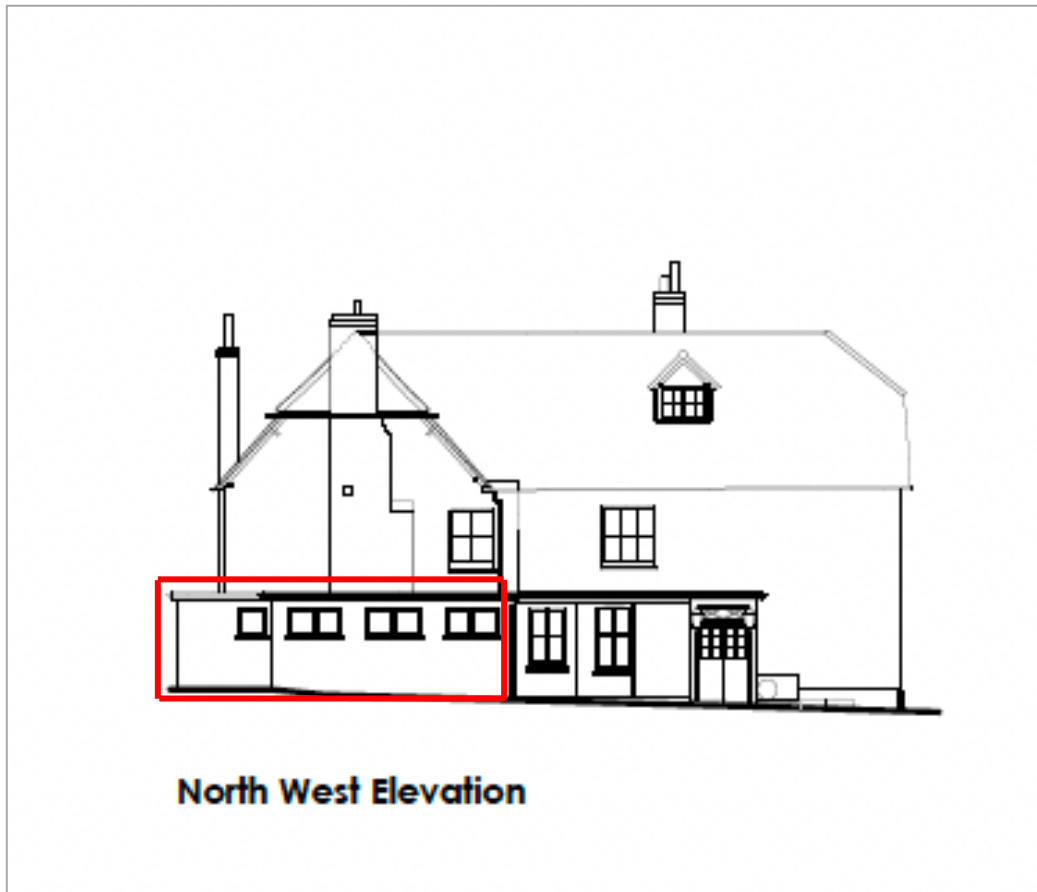
Figure 2. Toilet block demolished 2022 outlined in red
