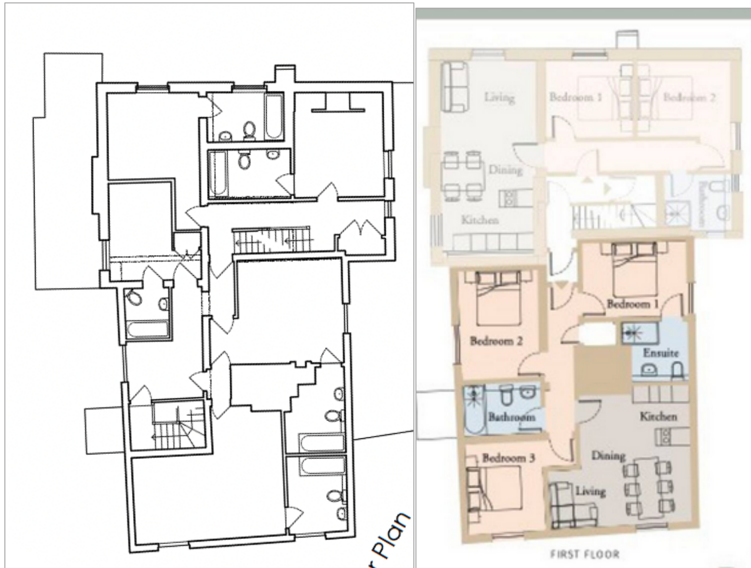
Figure 7. PRE-2022 First Floor The Queens Hotel 2022 LHS 5 en suite double bedrooms (10 bed spaces)- CURRENT 2024 RHS 2 self-catering apartments 5 double bedrooms (1 en suite) (10 bed spaces)
