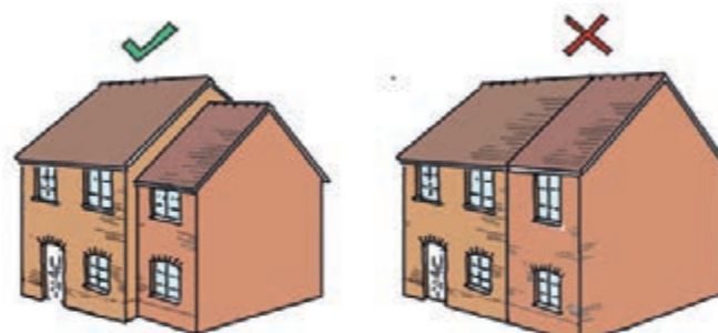
Figure 4.6: Extension should normally be set back from main house to retain latter's form and dominance and avoid mismatch of materials, except where appearance and symmetry can be improved.
