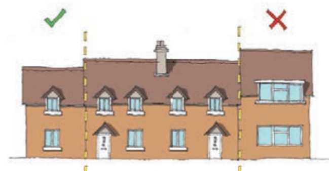
Figure 4.8: Keeping the ridge and eaves of an extension lower than the main building and maintaining the same roof pitch will help the original house maintain its dominance.
