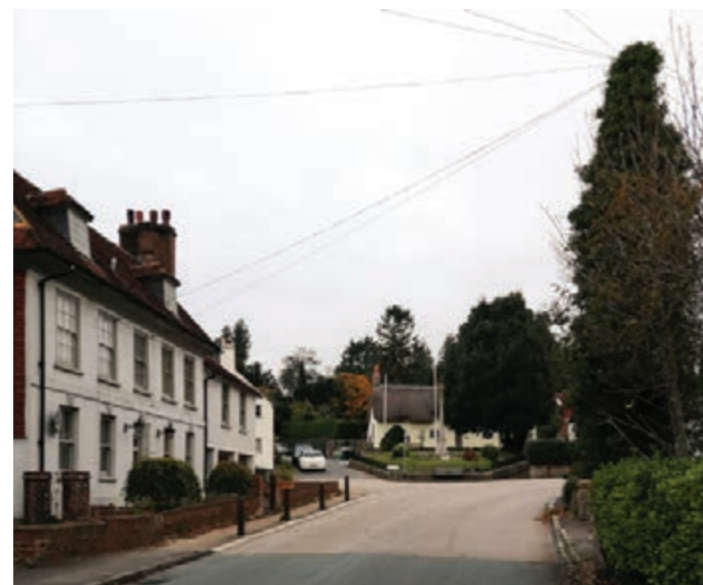
Figure 7.2: The A32 changes its surface treatment as it enters the centre of West Meon to signal to drivers that this is a zone where pedestrians can be expected.
