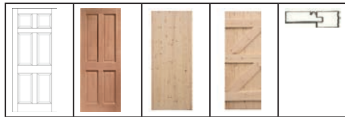
Figure 13.22: 6 and 4 panelled doors.
