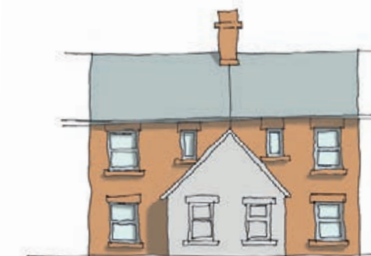
Figure 4.10: Traditional paired outshot extension to rear of terraced houses.
