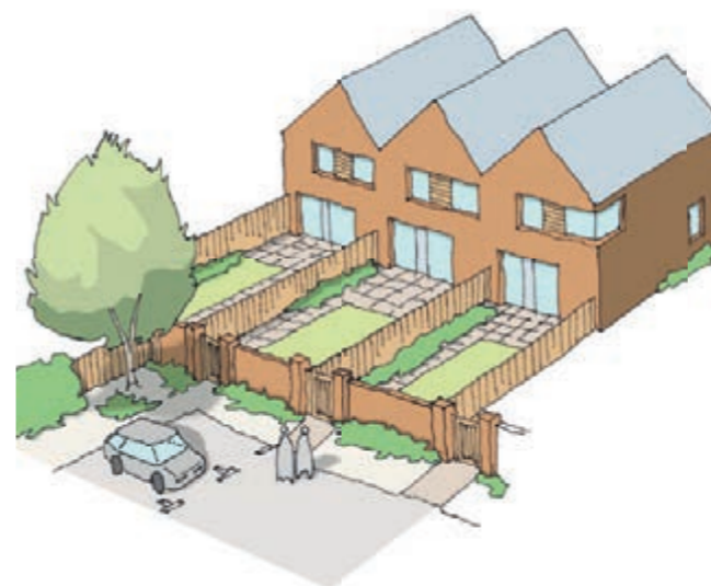
Figure 11.3: Rear gardens backing onto car parks, where unavoidable, should be in brick or stone with planting where possible.
