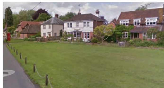
Figure 11.12: Post and chain boundary to village green used at Cheriton is traditional but can get visually dominant if on a large scale and does not invite spontaneous use.
