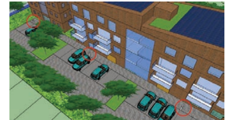
Figure 8.27: Illustration of how EV charge points could be located for flats (ringed in red).
