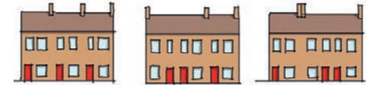
Figure 13.32: Three versions of a three house terrace showing the variations in chimney positions.
