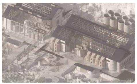
This project proposes utilising Waste Chalk Filter Cake (WCFC, spoil from chalk tunnelling) as the primary construction material. WCFC is used for chalk grassland regeneration and infilling of quarries, but can it be used for the renovation of buildings? And for bringing the industrial site back to life? How might an alternative construction curriculum emerge?
