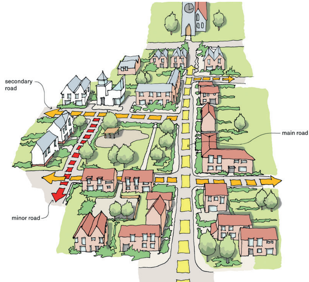
Figure 10: Elements of a Legible Development Showing Street Hierarchy (PUSH Quality Places model)
