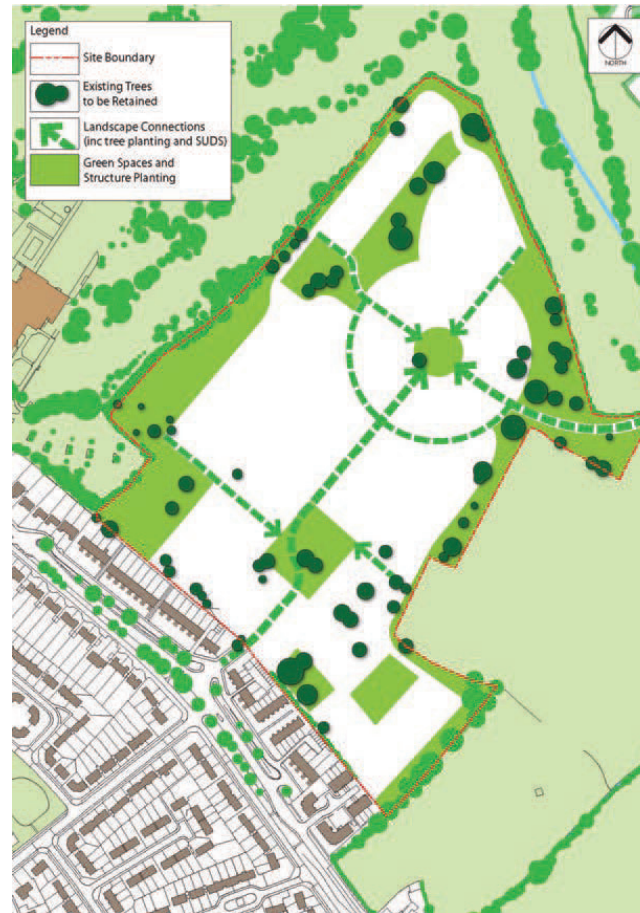
Figure 6: An Example of a Landscape Strategy is Expressed in a Landscape Framework Plan (Exeter Design Guide)
